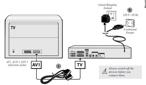
RGB-compatible scart/peritel cable (21 cabled pins).
